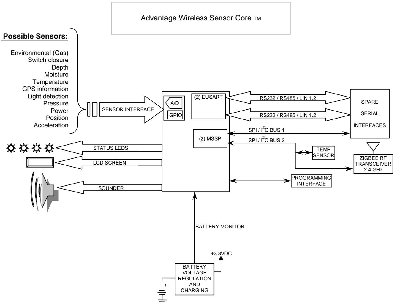
**Figure 1: Wireless Sensor Core™ Block Diagram**
